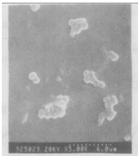
Fig. 2 Scanning electron micrographs of the surface of PTMG-H-N-I bead after contact with a Staph-aureus suspension
